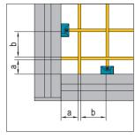
Note: The distance (a) between the nearest meshes and profiles have to be more than 20mm and less than b+5mm (b is the distance of the meshes). And the optimum distance between mounting blocks is 300mm to insure the structure intensity. 备注: 网丝与型材间距a需满足20mm<a<b+5mm (b为该网的网格距离寸)建议 螺母块安装间距300mm以确保安装强度。
